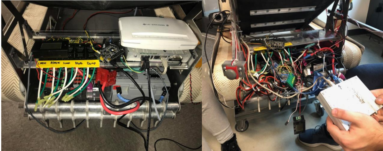
Figure 13: IBEX Control System Before and After 2018 Competition
